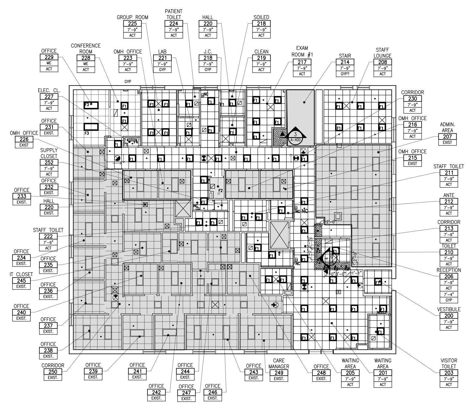
SECOND FLOOR REFLECTED CEILING PLAN SCALE: 1/8" = 1'-0"
